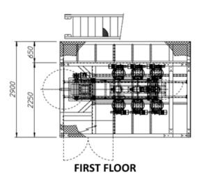
The system is customizable: starting from an evaluation of the types of production, Compact can be equipped with a different numbers of color dosing station (from 1 to 6). It can be integrated with the existing production lines, upstream the presses, that will be directly loaded with colored powder, and it guarantees an interconnection with the existing electrical boards.
