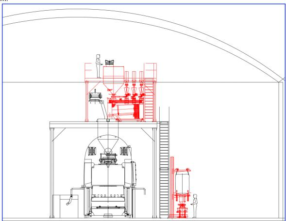
Ground positioning with pigments manual loading hopper:
